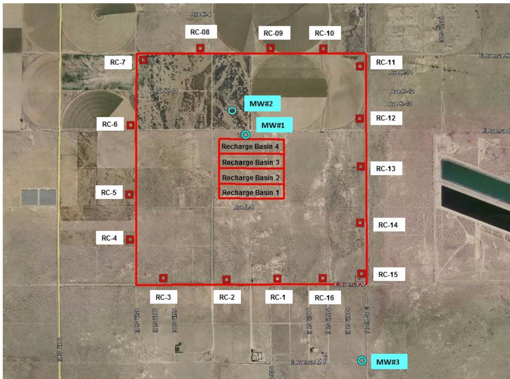
Figure 10-3: Monitoring and Recovery Well Locations
